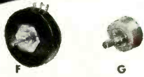
MODELS F AND G PRECISION SINGLE-TURN POTENTIOMETERS Feature both continuous and limited mechanical rotation, with maximum effective electrical rotation. Versatility of designs permit a wide variety of special features. F—3-5/16" dia., 5 watts, electrical rotation 359°—resistances 10 to 100,000 ohms. G—1-5/16" dia., 2 watts, electrical rotation 356°—resistances 5 to 20,000 ohms.
