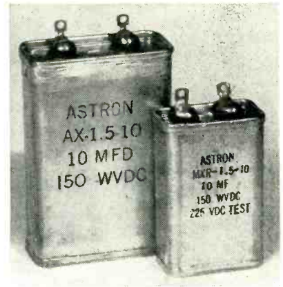
Comparison of sizes of 10- \mu f, 150 wvdc hermetically sealed paper capacitors with conventional (left) and metallized construction
