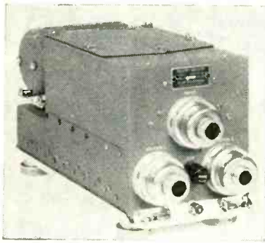
Packaged design permits addition of selective isolation amplifier to existing aircraft systems
