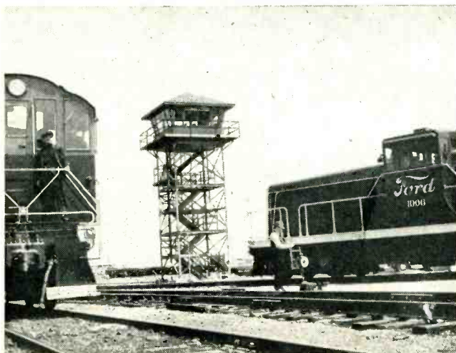
Dispatcher (right) at the mike of Ford railroad's new radiotelephone communication system relays switching orders to diesel locomotives in the 105-mile track yard. The traffic direction unit is located in a 42-foot high control tower (left)
