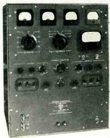
Precision phasemeter gives phase difference of two sinusoidal voltages directly in degrees
