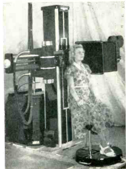
British cineradiograph apparatus. X-ray tube is in housing at patient's right. Fluorescent screen and 35-mm camera are on patient's left
