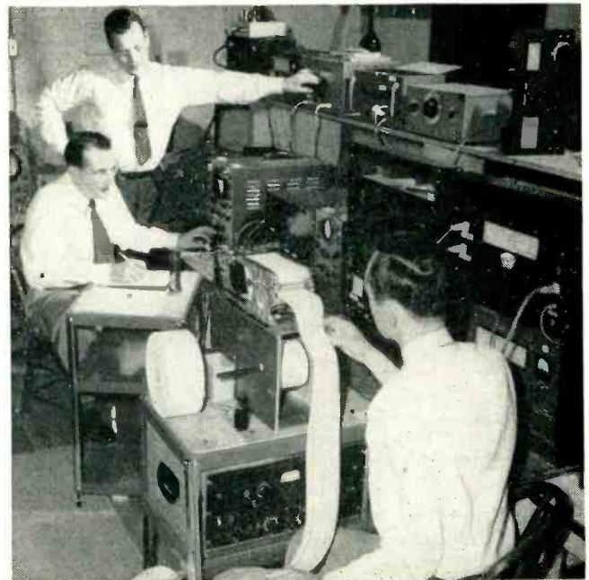
Doppler beats between transmitted and reflected c-w signals are recorded on tape to furnish wind-velocity data
