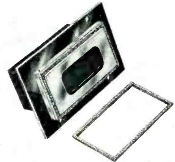
A Sylvania Electric TR tube showing Metex gasket loose and in position
